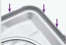
No dents in rim of the container lid Aluminium lid not warped
