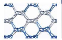
Material: Polypropylene, knitted monofilament
