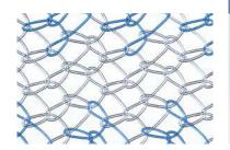
Material: Polypropylene, knitted monofilament
